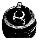
Overheated plug indicated by burned or blistered insulator tip and badly worn electrodes. This condition may be caused by preignition, cooling system defects, lean air/fuel ratios, low octane fuel, or over advanced ignition timing.
