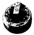
Oil fouling indicated by wet, oily deposits. A hotter plug temporarily reduces oil deposits but a plug that is too hot leads to preignition and possible engine damage.
