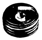
Normal plug appearance noted by the brown to grayish-tan deposits and slight electrode wear. This plug indicates the correct plug heat range and proper air fuel ratio.
