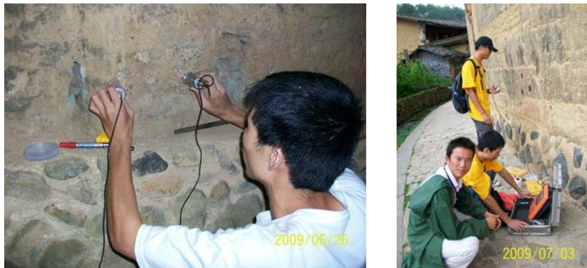
Fig 7: Ultrasonic testing heads and device
