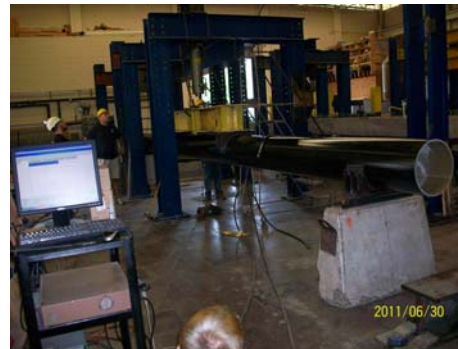
Figure 11 A 16" diameter FRP pipe being tested at CFC-WVU Laboratory
