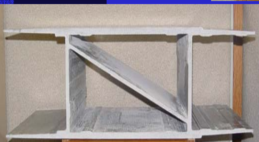
3. Lightweight composite bridge deck
