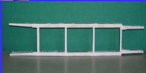
4. Low profile bridge deck
