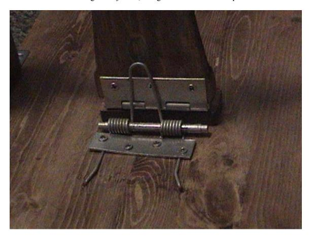
On our first prototype of the catapult, several things went wrong. First off, the top of the arm was designed in the shape of a "U". With this arm we had planned on placing a pouch inside the "u" to hold the golf ball.
