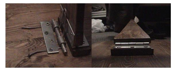
By changing the base of the arm and allowing it to go back farther, we also eliminated the high trigger mechanism, enabling the fulcrum to be locked in place with the spring fully compressed.
