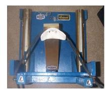
Below, we have constructed a graph that lays out a series of test runs that we preformed to test and alter the accuracy of our catapult. Our test runs contained a range of different number; this was the result of constantly altering the cross bar and tension on the radial arm. First, altering the cross bar gave us the ability to change the angle at which the ball was released.
